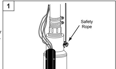
**CAUTION:** Be sure the top edge of the well casing is perfectly smooth. Sharp or jagged edges can cut or scrape the cable and cause a short. Do not let the cable drag over the edge of the well casing since this may cause damage to the insulation.
